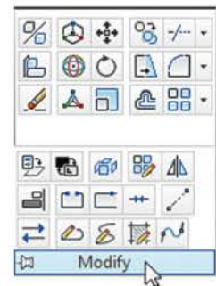
Fig. 6.1 The Modify tool icons in the Home/Modify panel
