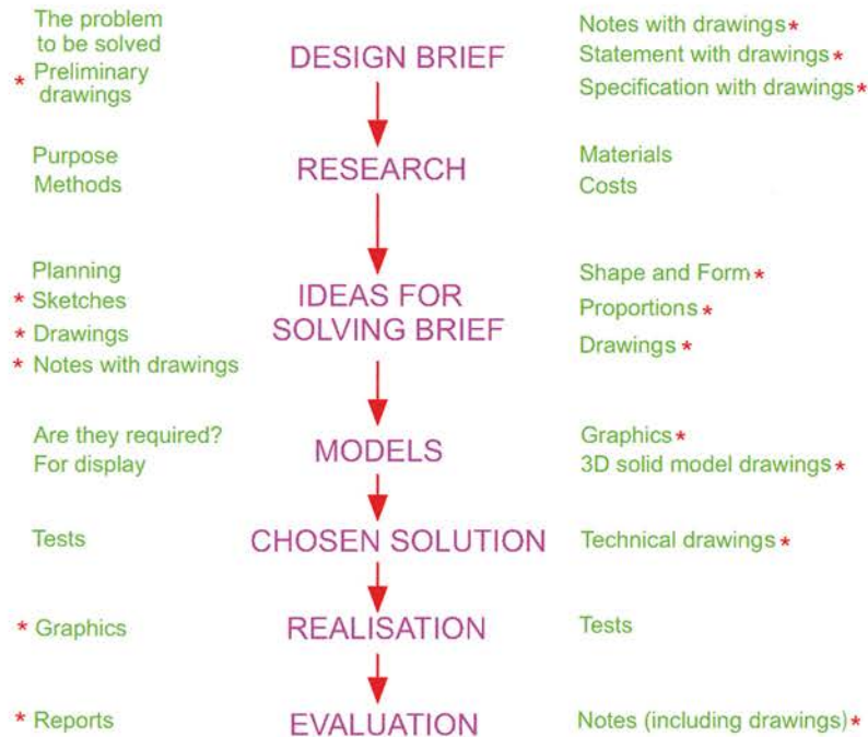
Fig. 21.1 A simplified design chart
