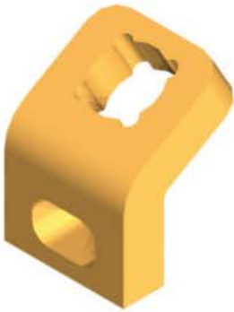
Fig. 18.25 Second example – 2D outlines in 3D space
