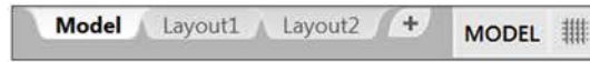
Fig. 1.18 The Model and Layout tabs on the left hand and the MODEL button in the status bar.
