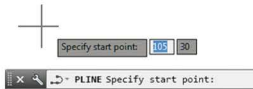
Fig. 2.3 What appears when Polyline is selected from the Draw panel
