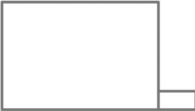
Fig. 17.16 First example – the four walls in their correct positions relative to each other in a ViewCube/Top view
