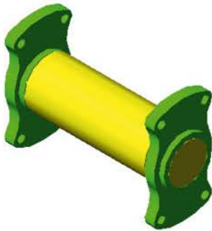
Fig. 14.27 Exercise 2 – a rendering of the holders and roller
